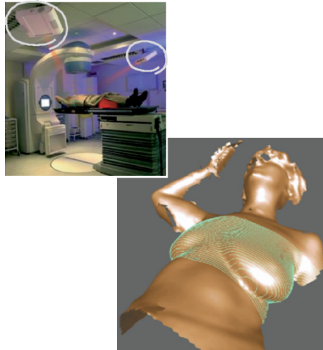
Figure 7.5. Top left: view of a treatment room outfitted with two (for a more complete view) stereo-photogrammetric cameras (outlined), and, bottom right, a projection view of a measured 3D skin surface with computed surface contour lines superimposed. Figure courtesy of Vision RT, Ltd.
